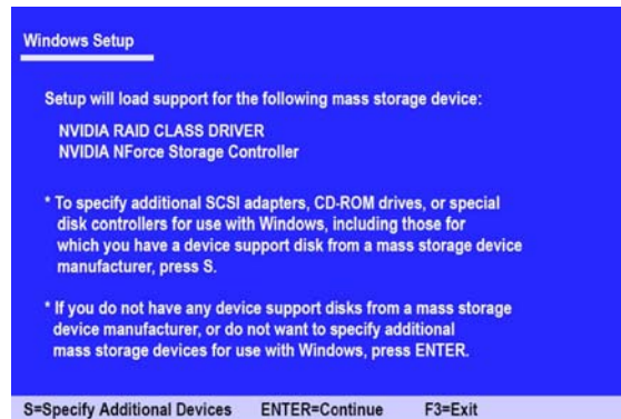
Figure 2.15 Windows Setup—NVIDIA drives listed
